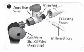
Locate the cold water line. Shut off the cold water supply. Unscrew the flexible supply line from the Angle Stop. Attach the Angle Stop Adapter (may look different than pictured). (Fits standard 1/2" and 3/8" plumbing with provided adapter.)
