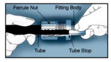
**NOTE:** It is not necessary to disassemble this fitting for application. Merely insert tubing to stop and tighten nut.
